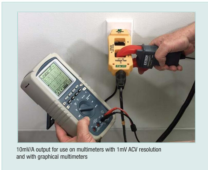
10mV/A output for use on multimeters with 1mV ACV resolution and with graphical multimeters
