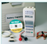
Includes software with cable, Kelvin alligator clips, Kelvin test leads, 6 AAA batteries
