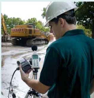
The PR20 Portable Thermal Printer gives you the means to document your pre- and post reading calibrations and the target noise source.
