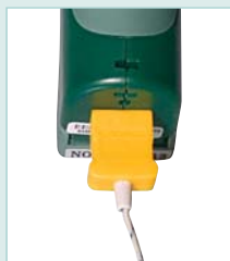
Type K input for contact measurements
