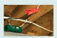
External NCV probe can be used to identify wiring in hard-to-reach areas where the transmitting unit cannot fit
