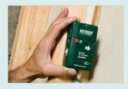
Clamp-on unit will sense AC Voltage of a mid-run wire and transmit the voltage present signal to the receiver indicator unit.
