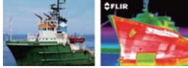
Boat - An IR camera can detect alterations made to vessel structure. Image shows a plate welded to the hull.
