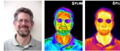
Graph 1.1 Visible photograph and two infrared thermograms, one with a rainbow palette and the other with an iron bow palette.
