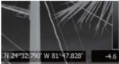
Graphs 4.11a Camera automatically adds position data to each IR-image
