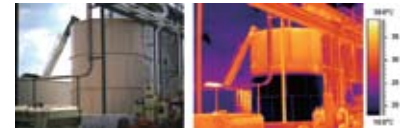
Liquid storage tank - An IR camera can show when there are multiple levels in a tank, allowing workers to determine whether or not the product is contaminated or the tank itself needs to be serviced. This allows them to optimize the product. And when weather conditions are optimal, leaks from PRV's, steam, hot gases and propane can be illuminated.
